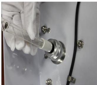
**Step 9:** Plug the ballast cable into the UV lamp. Install the cover cap and fit washer and earth wire using the pinwheel screw.
