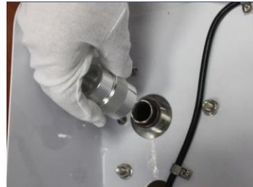
**Step 8:** Insert the spring into the Quartz sleeve and carefully insert the UV Lamp into the Quartz sleeve through the top nut.
