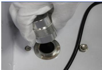
**Step 4:** Insert the Quartz sleeve into the Reactor Chamber.
