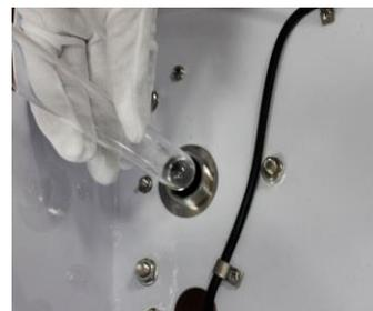
**Step 5:** Fit O-ring to bottom of Quartz sleeve as shown then screw bottom nut tightly onto chamber using your hand.
