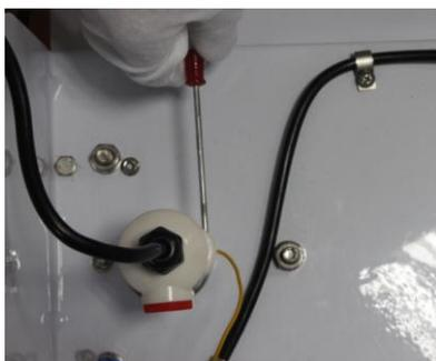
**Step 10:** Install the earth wire to the base.
